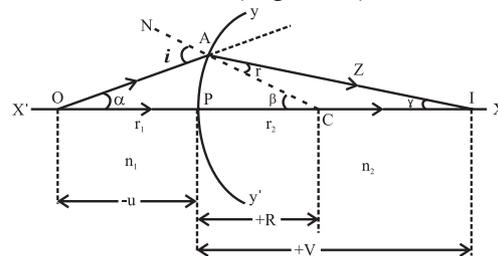
Fig. 9.12: Refraction at a single refracting surface.
