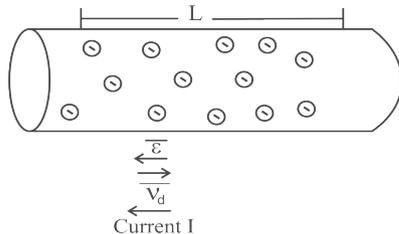
Fig. 11.3: Conducting wire with the applied electric field.
