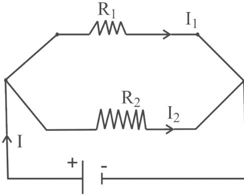
Fig. 11.10 : Two resistors in parallel combination.
