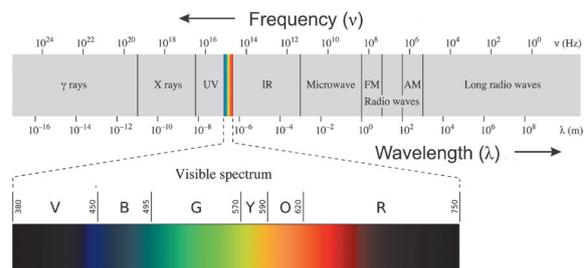
**Fig. 13.2: Electromagnetic spectrum.**
