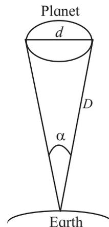
Fig. 1.4: Measurement of size of a planet
