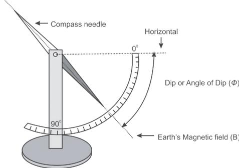
Fig. 12.7: Magnetic inclination.
