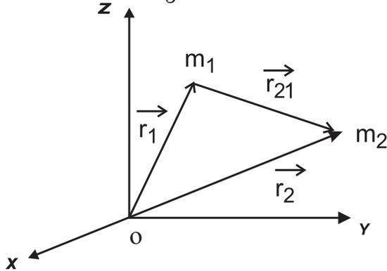
Fig. 5.3: Gravitational force between masses  $m_1$  and  $m_2$ .
