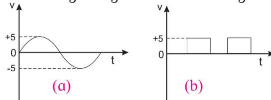
**Fig 13.7: (a) Analog signal. (b) Digital signal.**
