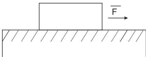
**Fig. 6.10: Static friction.**
