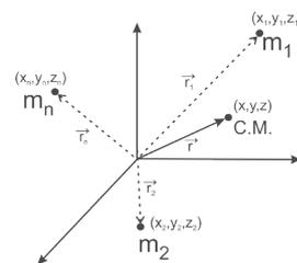
Fig. 4.11: Centre of mass for  $n$  particles.
