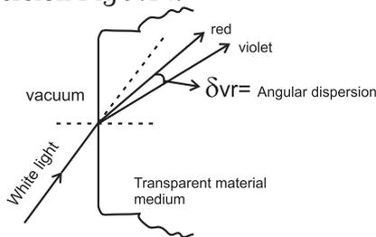
**Fig. 9.14: Angular dispersion at a single surface.**
