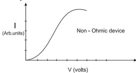
Fig. 11.5:  $I$ - $V$  curve for non-Ohmic devices.
