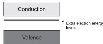
**Fig.14.11: Schematic band structure of an n-type semiconductor.**
