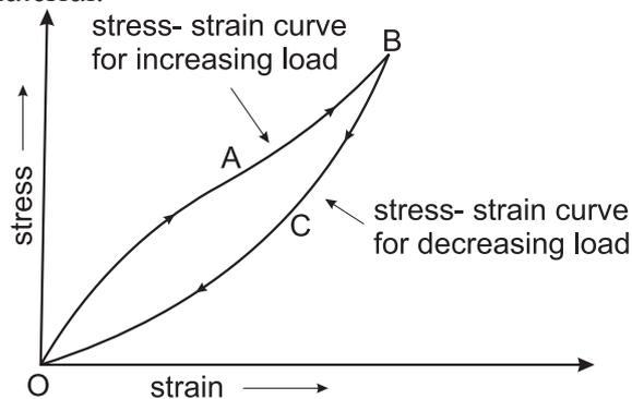
Fig. 6.8: Stress-strain curve for increasing and decreasing load.
