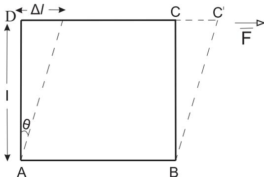
Fig. 6.3 : Tangential force produces shearing stress.
