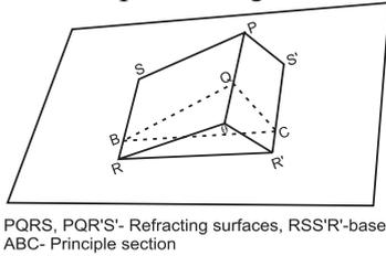
Fig. 9.16: Prism consisting of three plane surfaces.
