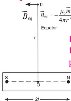
Fig. 12.2 (b): Magnetic field along the equatorial point.
