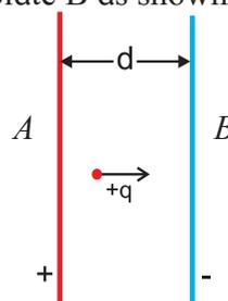
Fig 10.10: Electric field between two parallel plates.
