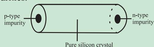
The impurities grow on either side of the crystal after heating in a furnace. Electrons and holes combine at the center and the depletion region develops. A junction is thus formed. Electrodes are inserted after cutting transverse sections and hundreds of diodes are prepared. All semiconductor devices, including ICs, are fabricated by 'growing' junctions at the required locations.
