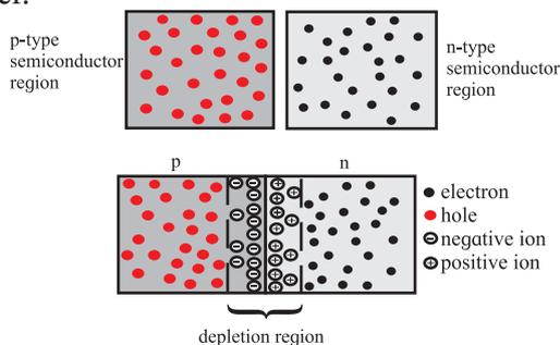
Fig. 14.17: Potential barrier and the depletion layer.
