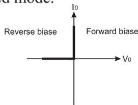
Fig. 14.27: I-V characteristics of an ideal diode.
