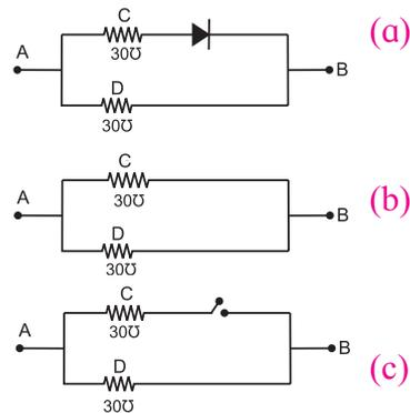
**Solution:** We know that for an ideal diode, the resistance is zero when forward biased and infinite when reverse biased.
