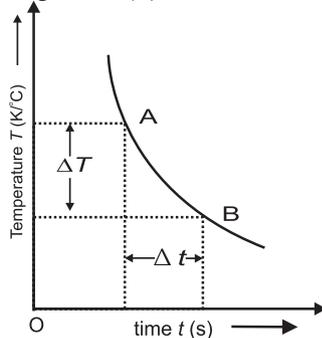
**Fig 7.13 (a):** Temperature versus time graph.  $\lim_{\Delta t \rightarrow 0} \frac{\Delta T}{\Delta t}$  gives the slope of the tangent drawn to the curve at point A and indicates the rate of fall of temperature.
