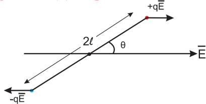
Fig. 10.19 (b): Couple acting on a dipole.
