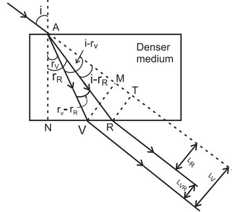
**Fig. 9.15: Lateral dispersion due to plane parallel slab.**
