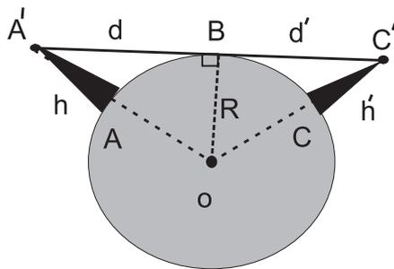
Fig. 13.5: Range of the signal (not to scale).
