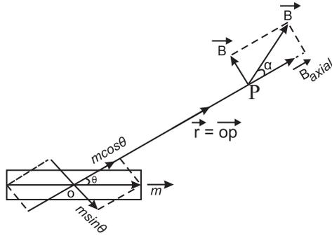
Fig. 12.3: Magnetic field at an arbitrary point.
