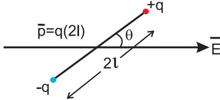
Fig. 10.19 (a): Dipole in uniform electric field.
