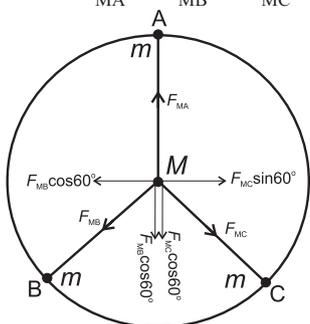
Forces  $F_{MB}$  and  $F_{MC}$  are resolved along  $F_{MA}$  and perpendicular to  $F_{MA}$  as shown. Components perpendicular to  $F_{MA}$  cancel each other. Components along  $F_{MA}$  are
