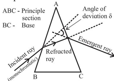
Fig. 9.17 (a): Refraction through a prism (monochromatic light).
