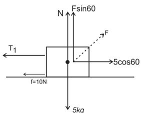
Fig 4.2 (c): Free body diagram for 5 kg mass.
