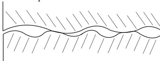
Fig. 6.9: Microscopic view of polished surfaces in contact.
