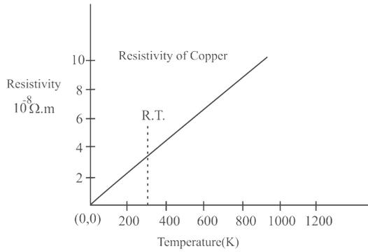
Fig. 11.11: Resistivity as a function of temperature (K).
