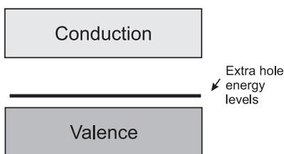
Fig. 14.14: Schematic band structure of a p-type semiconductor.
