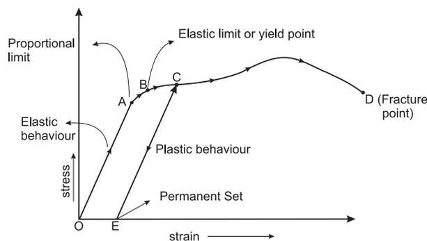
Fig. 6.7 : stress-strain curve.
