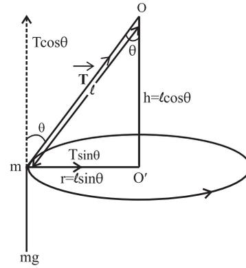
Fig 3.7: Conical pendulum
