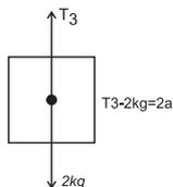
Fig 4.2 (b): Free body diagram for 2 kg mass.
