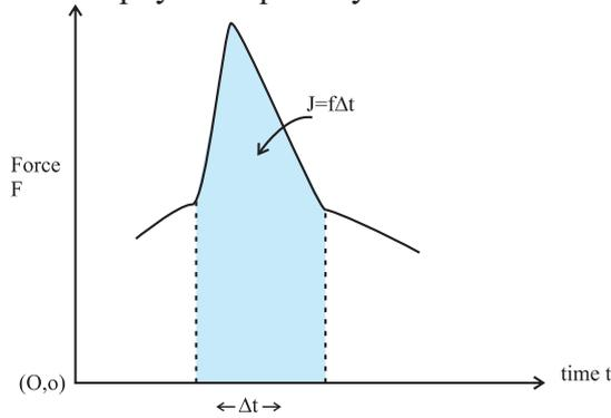
**Fig. 4.5:** Graphical representation of impulse of a force.
