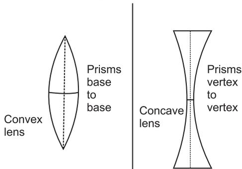
Fig. 9.23: (a) Convex lens (b) Concave lens
