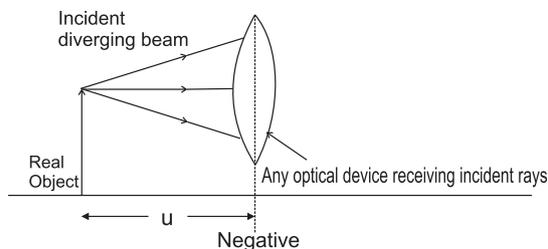
Fig. 9.2: (a) Diverging beam from a real object
