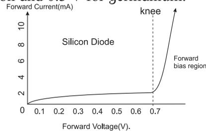
Fig. 14.24: I-V characteristic of a forward biased diode.
