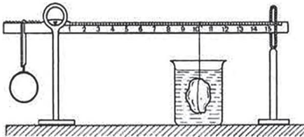
The reading 'Wa' is recorded by the position of sample in air, on the beam. The specimen is then immersed in water in beaker and is moved along the beam, until the constant weight is again counterbalanced and second reading 'Ww' is obtained. The reading 'Wa' and 'Ww' are inversely proportional to the actual weight of the body in air and water respectively.
